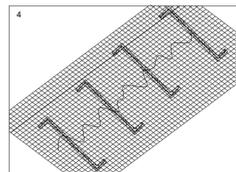
FIXAR TELA DE ARAME GALVANIZADO MALHA 4mm - FIO 22 90 cm - REBOCAR E PINTAR COM TINTA FLEXÍVEL
